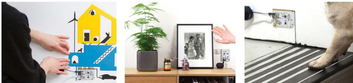
Figure 1. Touch-Board paint to create graphic sensors, objects as sensors, and sensing spaces [2]
